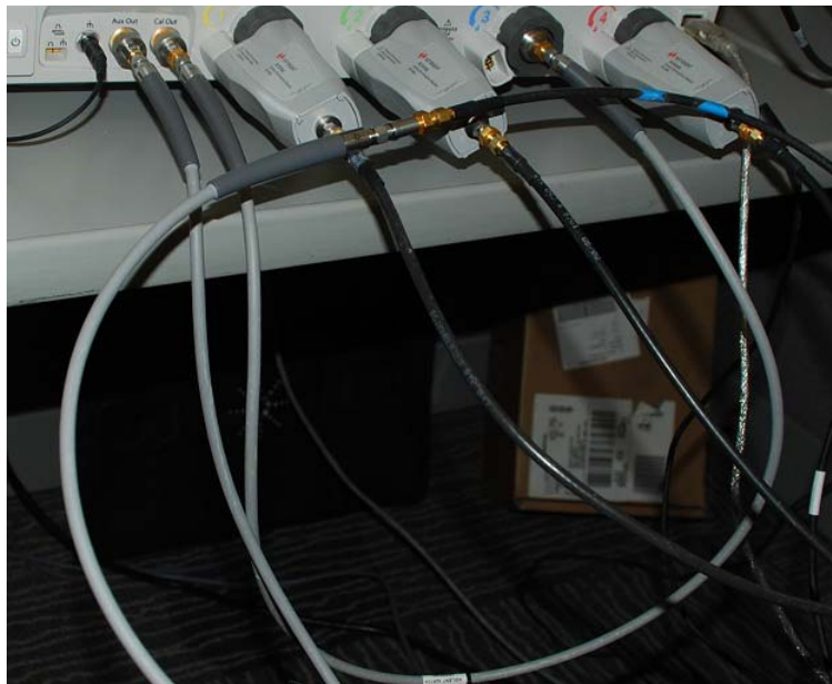
Figure 17 Connecting the Clk+ cable into channel 1, using the N7010A adapter
