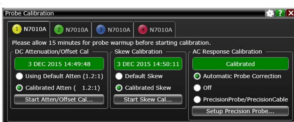
Figure 2 DC and Skew calcs completed
